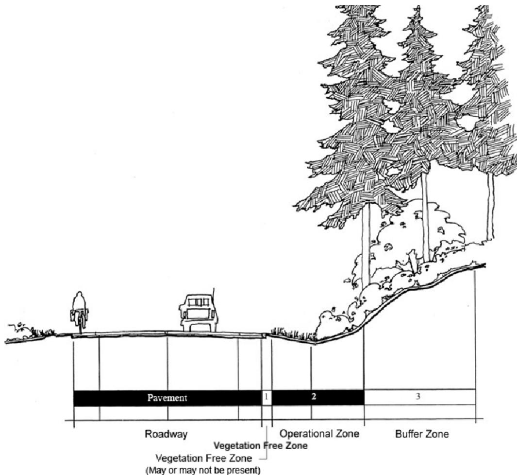
Figure 2. Right-of-way maintenance zones.
