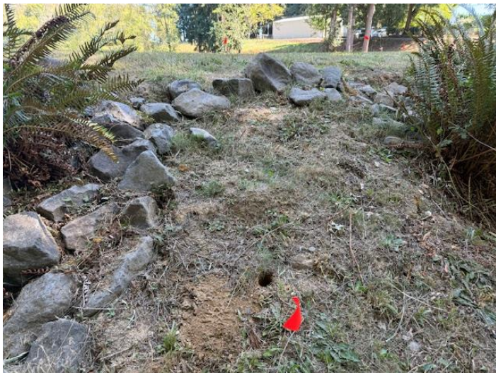
15. View of a typical sampling point (orange marker flag) from Earthen Dam, 1 of 10, composite sample: C4-Dam, with view of surface soils and imbedded cobbles. Sample area along western bank of the Dam, adjacent to creek culvert outfall area.
