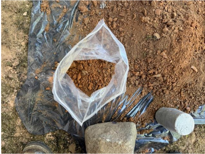
9. View of soils removed from 0 to 5.5 feet bgs on Visqueen, and from 5.5 to 6 feet bgs in ziplock bag prior to sampling west side of HOT; sample C5-HOT.
