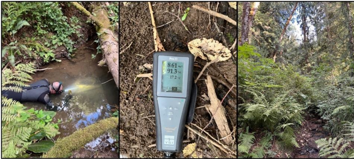
Figure 28. Pictures from a stream survey conducted on August 22, 2023 in Johnson Creek directly adjacent to PWB's proposed development site at Carpenter Lane. (left) Snorkel survey to confirm fish presence (center). Water quality measurements indicating suitable dissolved oxygen ( >8 mg/L) and summer temperature ( <18 °C) conditions for native cold-water fish species. Measurements taken at 17:00 PDT when stream temperature was at its daily peak. (right) Dense riparian vegetation surrounding the creek.
