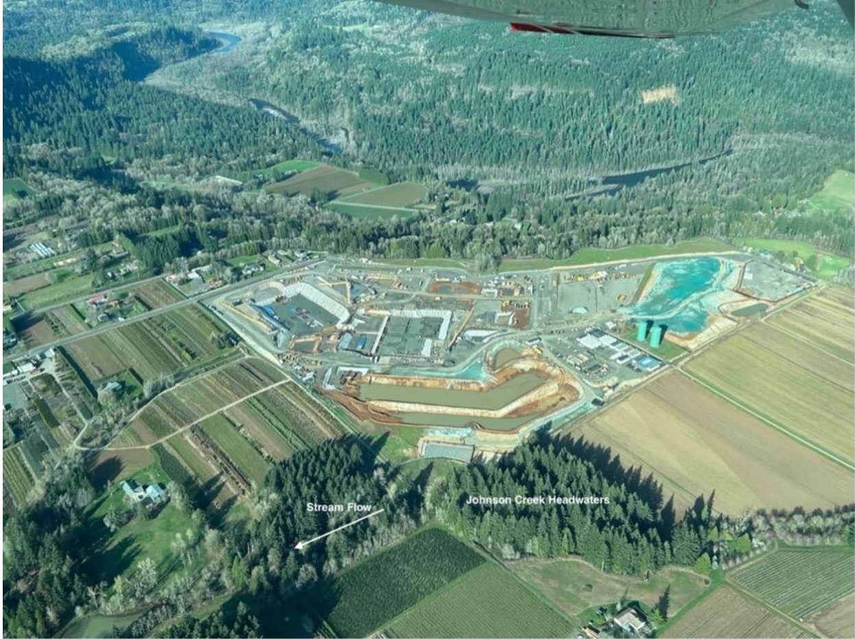
Figure 3. Aerial photo of the 90+ acre water treatment plant construction site (looking northeast) showing its proximity to Johnson Creek and the federally designated Wild and Scenic Sandy River. Stormwater collection and facility retention basins were intentionally sited 200 ft from the creek to facilitate discharge of excess storm water into the creek, away from the site. The creek is also currently being used to convey pumped groundwater from the local aquifer out from the construction site.
