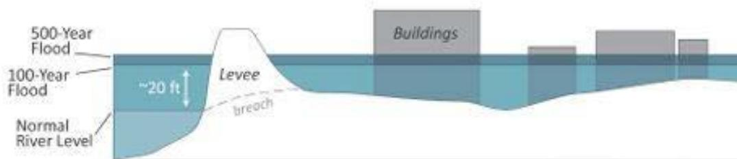
*Figure 59 - Graphic showing how a levee breach impacts buildings normally protected from high water. Graphic - DOGAMI.*
