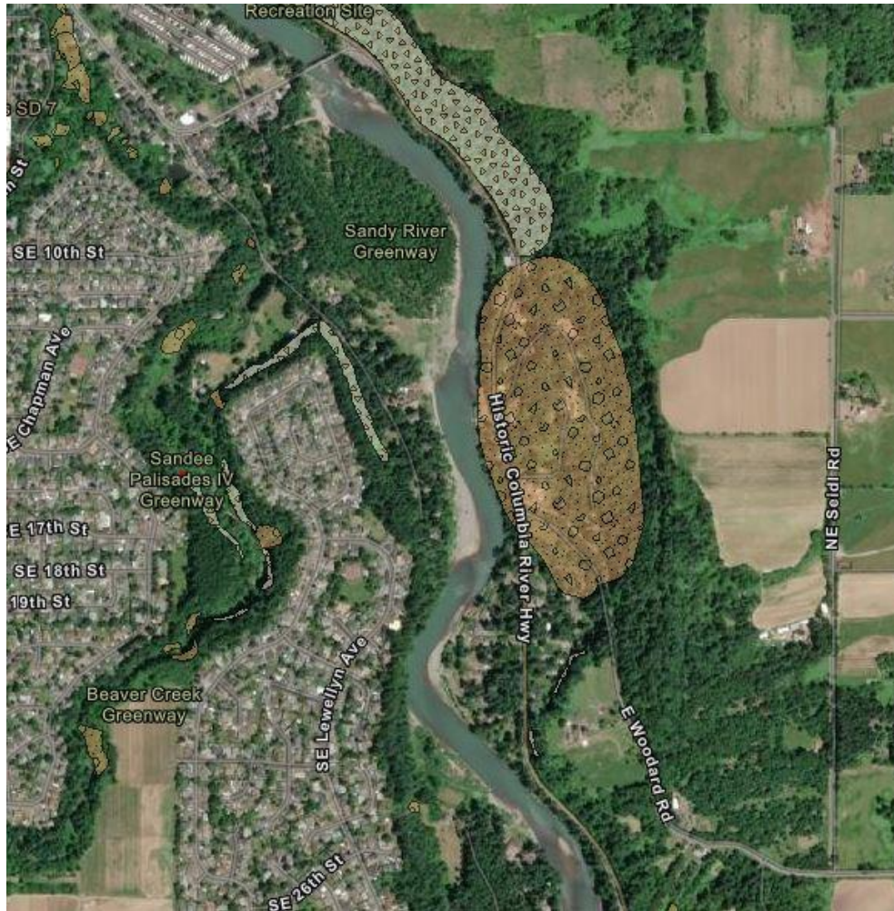
Figure 144- Map showing location of historic deep landslide deposits. The brown area is landslide deposit and the lighter color are rocky Talus-Colluvium deposits. Map from DOGAMI's HazVu site.
