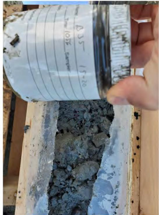
**Photo 24** - View of sonic core and soil subsample at in-water boring B-35.
