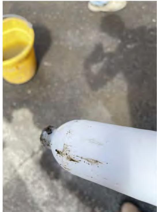
**Photo 16** - View of petroleum contamination encountered during groundwater sampling at boring B-18.
