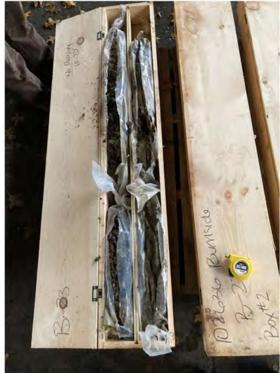
**Photo 12** - View of sonic cores from drilling at boring B-23.
