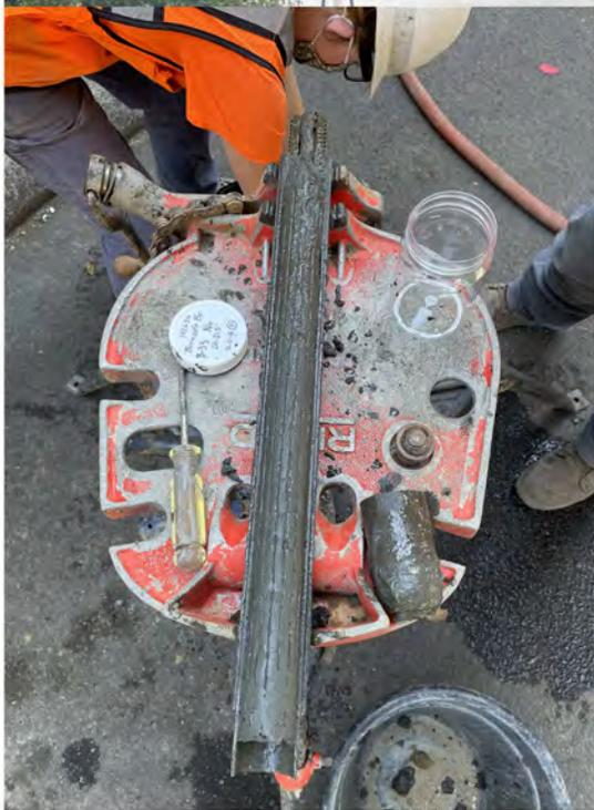
**Photo 21** - View of petroleum encountered at boring B-33.
