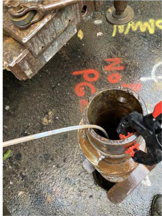
**Photo 2** - View of clogged groundwater sampling tubing at boring B-5.
