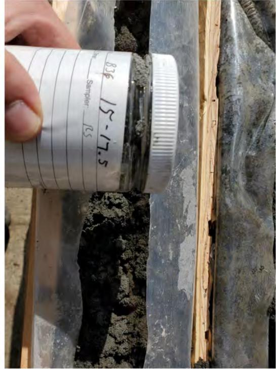
**Photo 30** - View of sonic core and soil subsample at in-water boring B-36.
