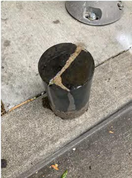
**Photo 19** - View of former roadway cobble encountered at boring B-20.
