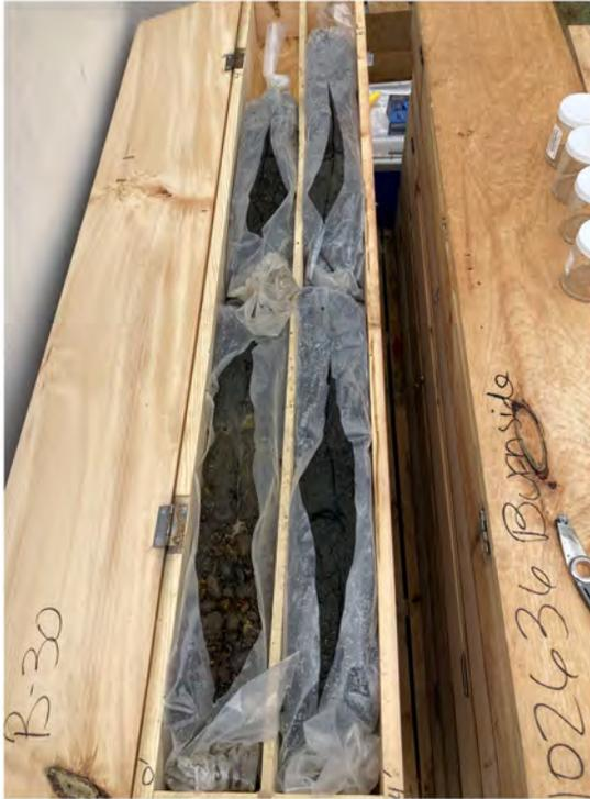
**Photo 29** - View of sonic cores from in-water boring B-30.
