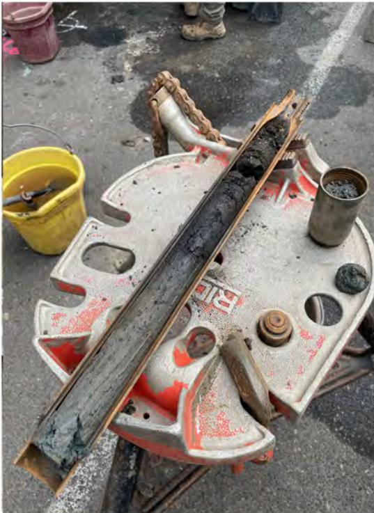
**Photo 15** - View of stained soil from boring B-18.
