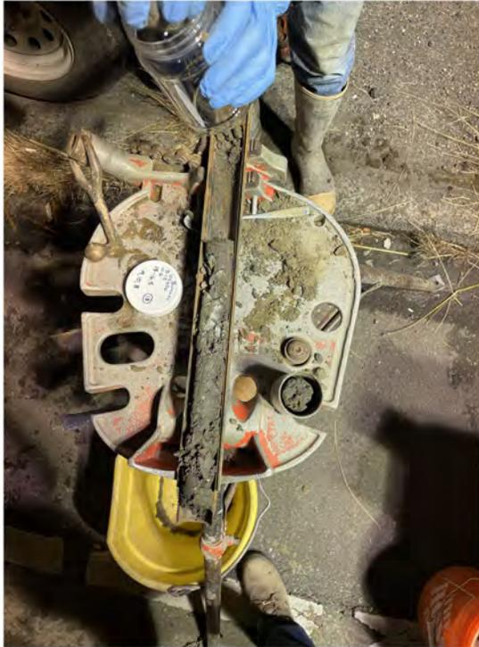
**Photo 13** - View of sample collected from boring B-15 along I-5 SB.
