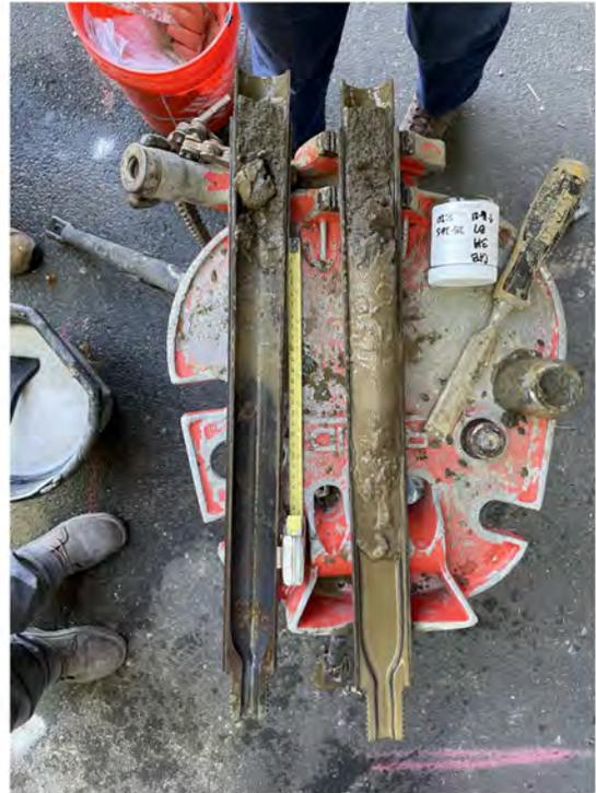
**Photo 4** - View of saturated sample from boring B-7 near SW Naito Pkwy.
