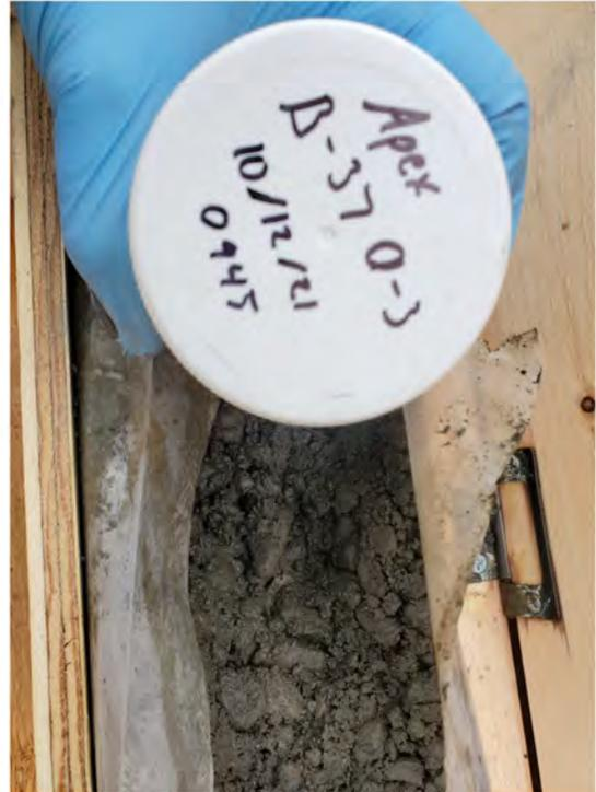
**Photo 32** - View of sonic core and soil subsample at in-water boring B-37.
