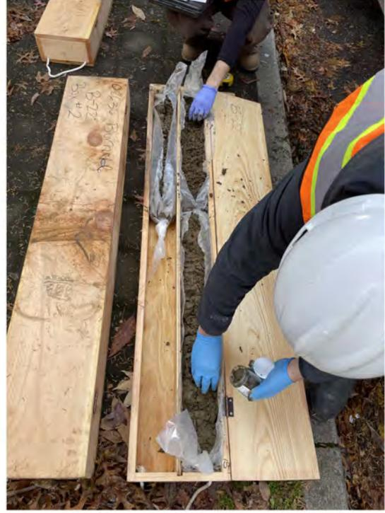
**Photo 10** - View of soil subsampling from boring B-22 sonic cores.
