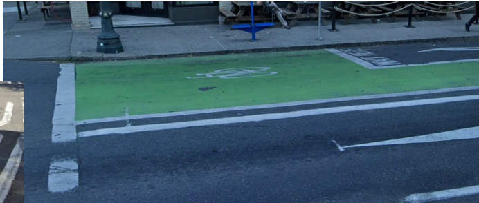
Top Right Image Description: Photograph bike box in front of curb-side right turn lane
