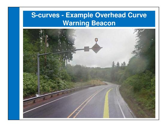
This is an example of an overhead flashing beacon and warning sign which we plan to construct on the uphill and downhill sides of the S-curves for better awareness of these being the most constrained curves in the corridor.
