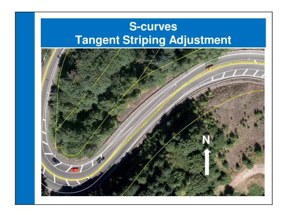
This is a more zoomed in picture of the previous slide showing the alignment change between curves. Note the difference between the striped centerline shown in the aerial photograph and the future yellow centerline drawn.
