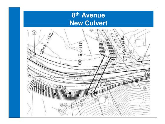
Since the project will be impacting an existing culvert in an historically fish bearing stream. federal requirements dictate we replace this existing pipe culvert with a much larger culvert to accommodate fish passage.
