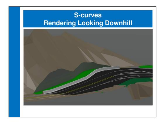
This is a computer generated rendering of what the improvements at the S-curves could look like from the uphill perspective. Notice the rock cut and rockfall area behind the concrete barrier.
