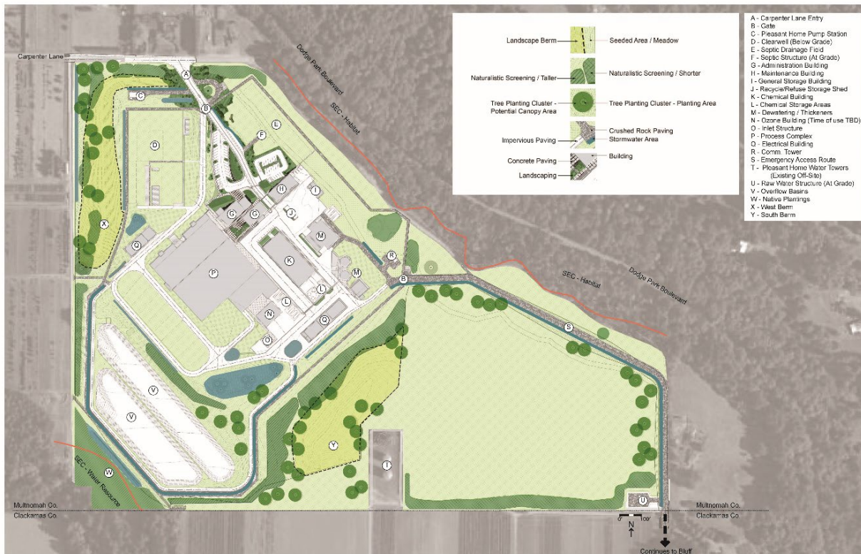
Figure 3. Filtration facility site with planted buffers and stormwater facilities
