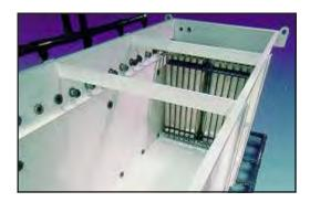
Membrane cartridges are placed into a basin.
