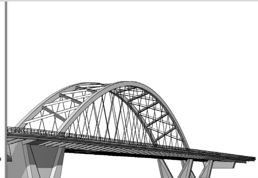
Braced vertical arches
