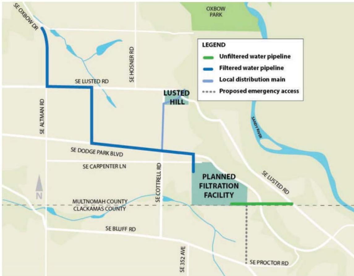
Figure 2. Location of the proposed Bull Run treatment facility showing the location of the various project components, including the Facility parcel (blue shading), the RW pipeline (green line), FW water pipeline (dark blue line), the Cottrell Road local transmission main (light blue line) to the existing Lusted Hill Treatment Facility, and the emergency access (grey dots) (from <https://www.portland.gov/ater/bullruntreatment/filtration/about>).
