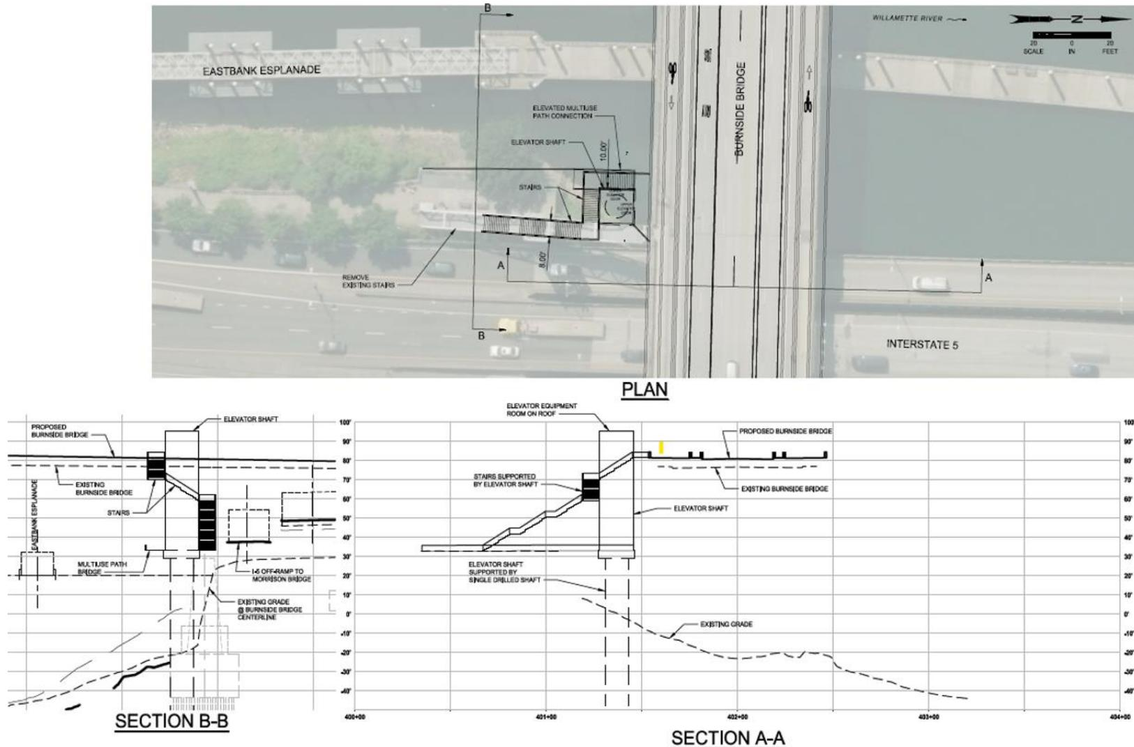
Figure 5. Ramps on North and South Sides of the Bridge and Stairs on South Side
