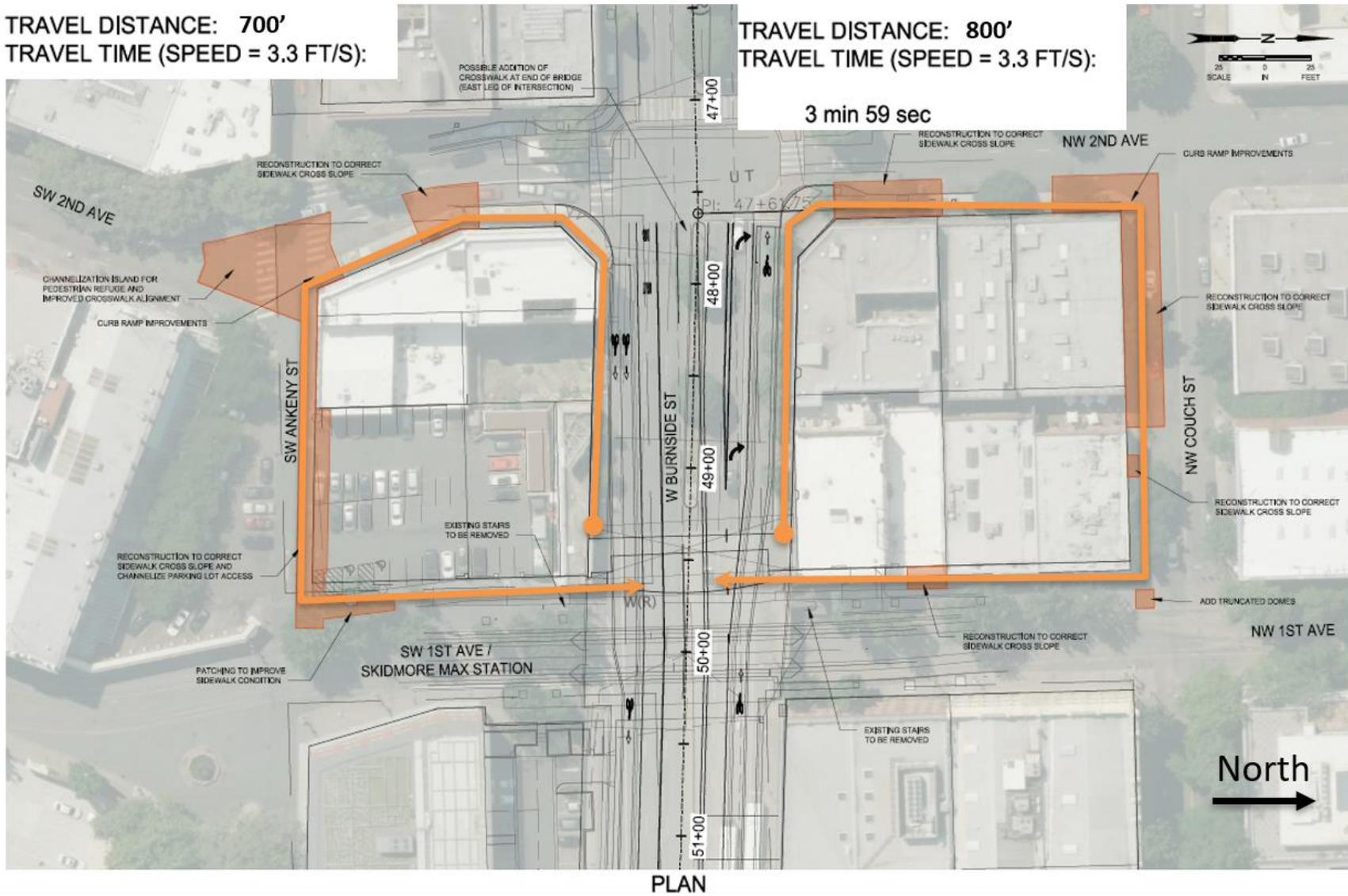
Figure 11. In-Kind Stairs on North Side; New Ramp (Mercy Corps Parking Site) and Stairs on South Side (Layout 1)
