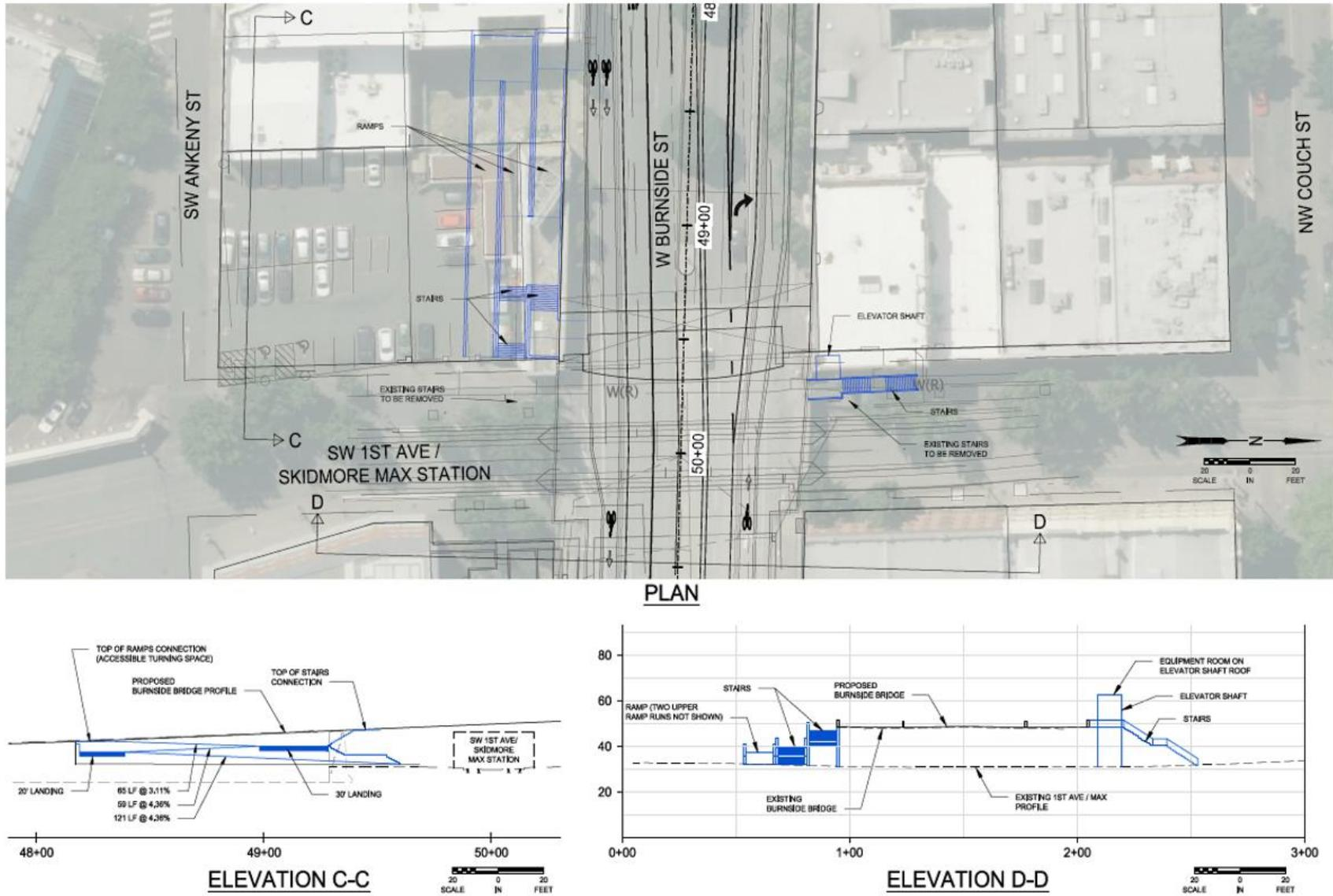
Figure 10. Sidewalk Improvement Routes from North Sidewalk (Point A) to Skidmore Foundation MAX Station (Point B)
