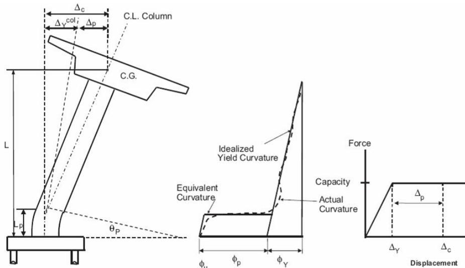
**Figure 11. Local Displacement Capacity – Framed Column, Assumed as Fixed-Fixed**
