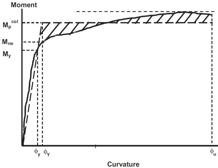
The ultimate curvature,  $\phi_u$ , is determined as the smaller of:
