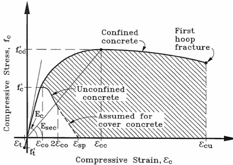
For modeling purposes, the unconfined concrete compressive strain at the maximum compressive stress shall be taken as  $\epsilon_{co} = 0.002$  (Guide Spec 8.4.4). The ultimate unconfined compression strain based on spalling shall be taken as  $\epsilon_{sp} = 0.005$  (Guide Spec 8.4.4).
