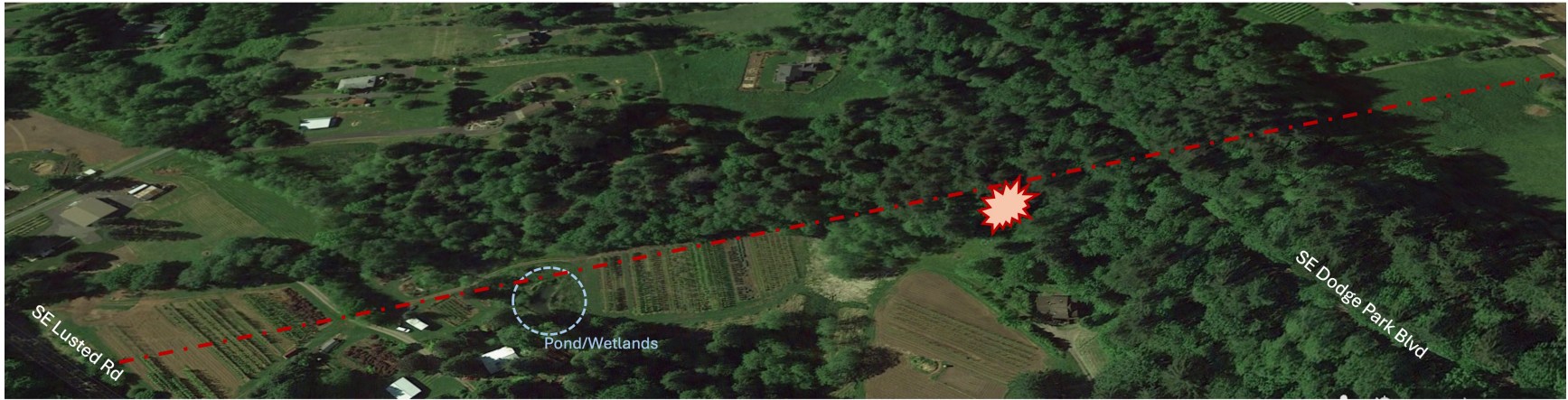
Figure 1. Estimated raw water pipeline (red hashed line) from Lusted Road conduit, facing southeast. Pipeline will extend through wetland habitat (blue circle) and toward portal within SEC-h (red blast icon) and continuing under the SE Dodge Park Blvd. Pipeline continues underground toward filtration site to the west
