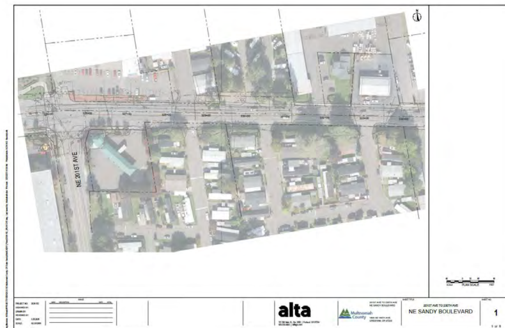
Figure 34. Surveyed Basemap Data including Digital Terrain Model and Features (Task 2.3), Preliminary Centerline and Preliminary ROW (Task 2.7)
