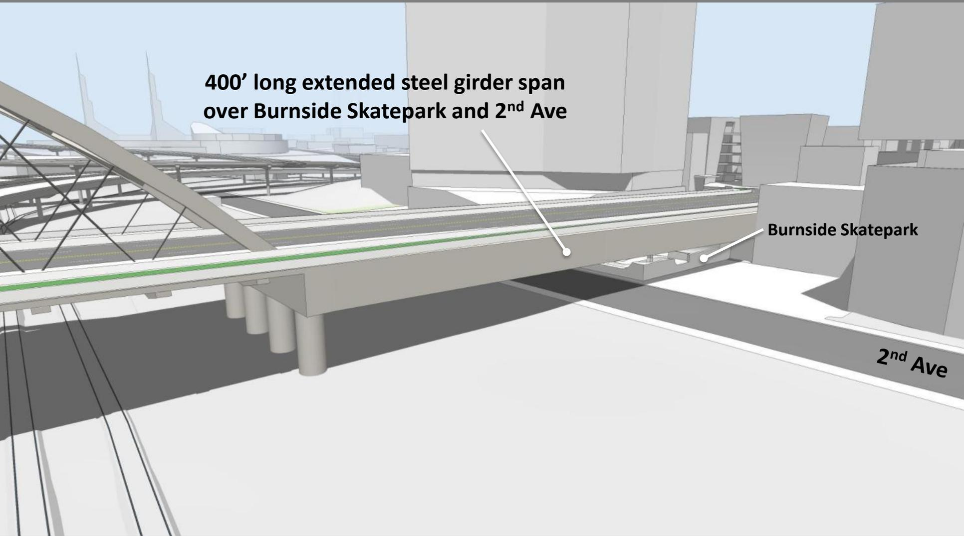
**400' long extended steel girder span
