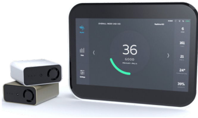
Figure 16: Air Quality Monitors.
