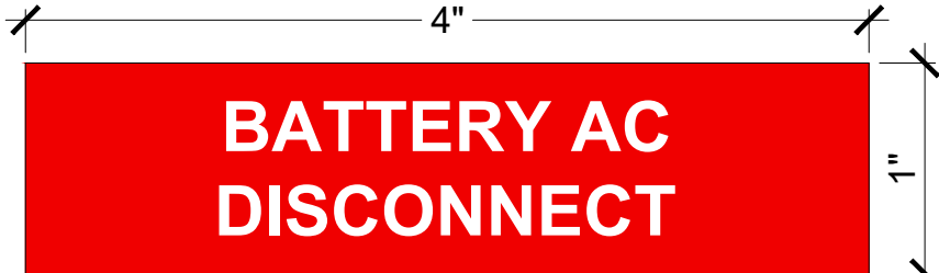
LOCATION: AC DISCONNECT QUANTITY:1
