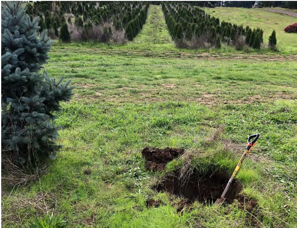
Photopoint 19: Plot 15 lies in an area of active nursery activity within the proposed filtration facility site. Soil was friable and well drained, and lacking indicators of wetland hydrology.
