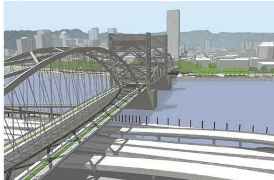
Long-span Alternative / Cable-stayed / Lift
