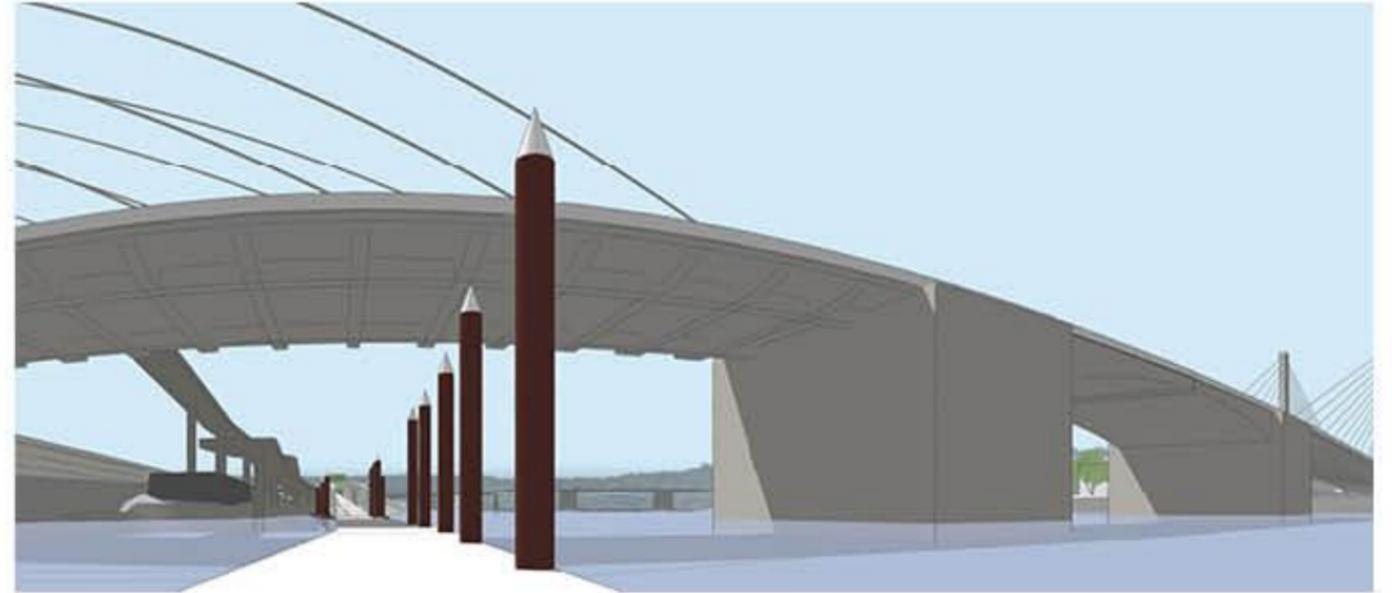
Long-span Alternative / Tied-arch / Lift\*
