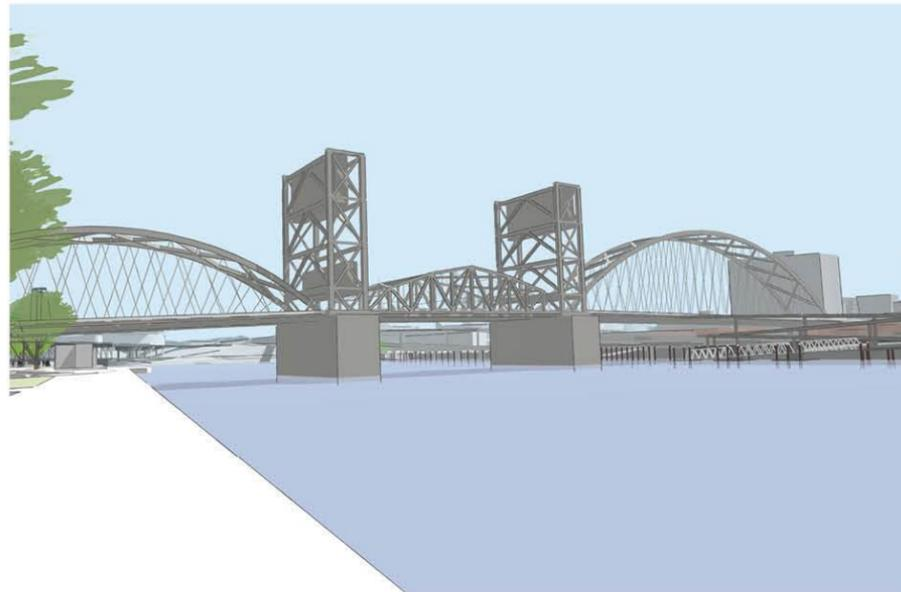
Long-span Alternative / Cable-stayed / Lift
