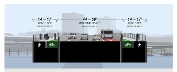
The project team proposes reducing the width of the bridge compared to the initial Preferred Alternative. The new bridge would be roughly the same width as the current bridge but with one less vehicle lane.
