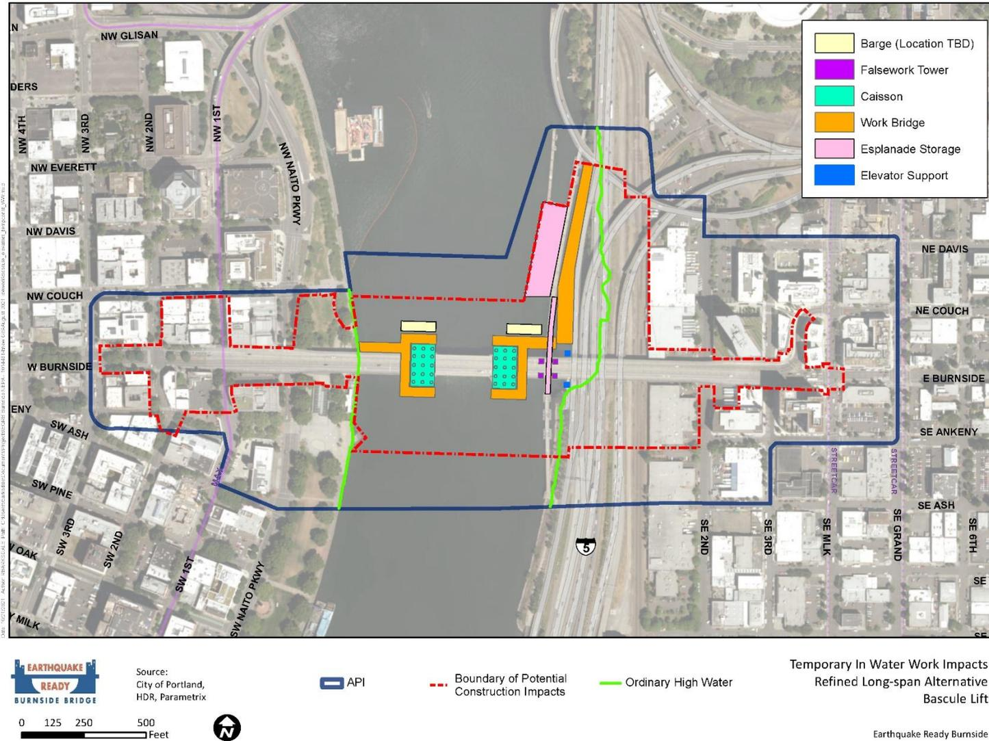
Figure 7. Temporary In-water Impacts Refined Long-Span Alternative with Vertical Lift
