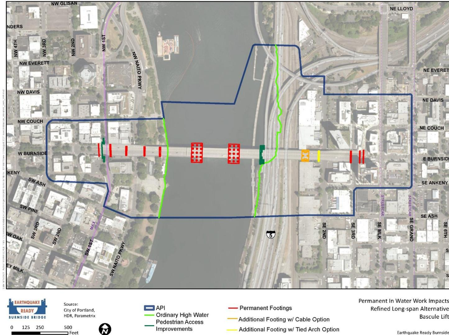
Figure 9. Permanent In-water Impacts Refined Long-Span Alternative with Vertical Lift
